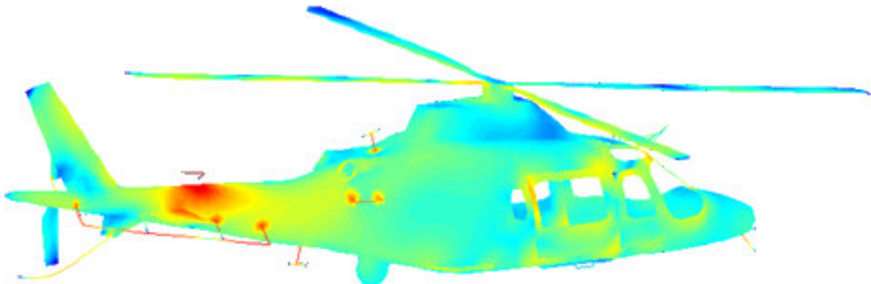
Figure 27: Induced Current Distribution at 108 MHz
